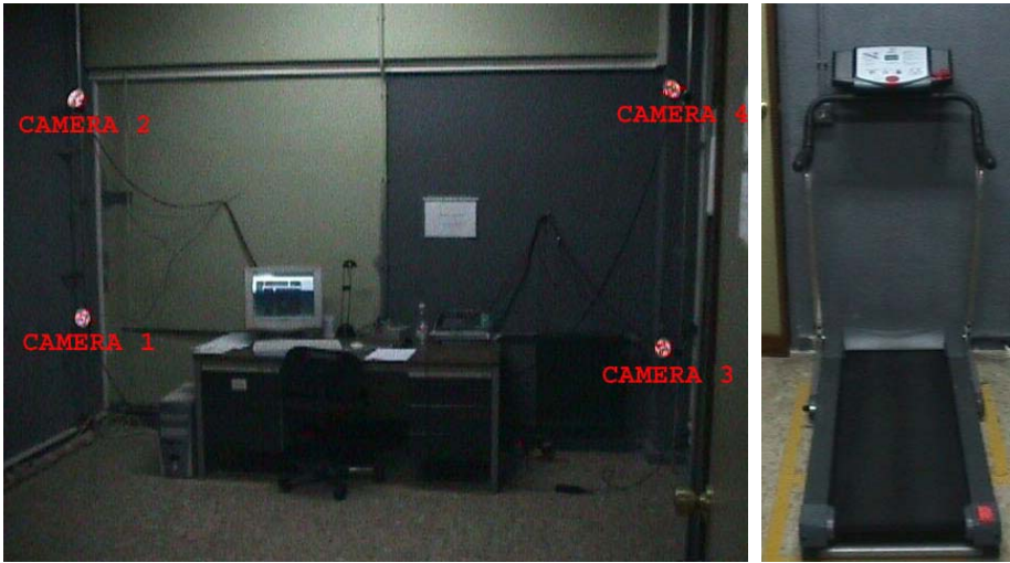
Fig. 1. Stereovision system composed by four cameras, frame-grabber and PC, and the conveyor belt
